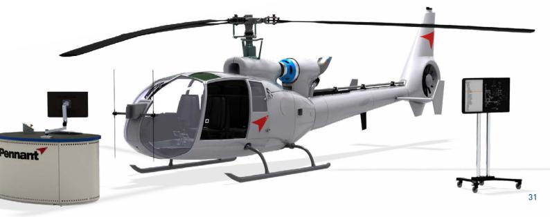
The Integrated Avionics Maintenance Trainer (IAMT) is an avionics part task trainer that enables practical avionics maintenance tasks to be taught by either instructor demonstration or independent, practical exercises for the student.
