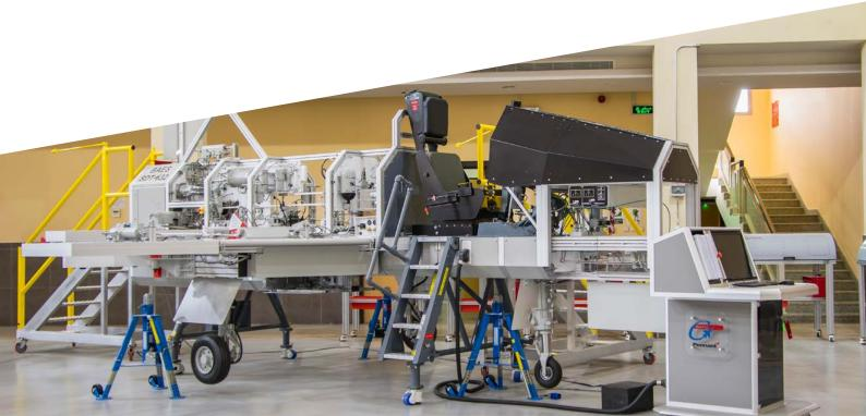
The Basic Helicopter Maintenance Trainer (BHMT) is a freestanding helicopter trainer enabling students to carry out practical training by performing standard maintenance procedures associated with rotary wing aircraft. There are many systems on which the student can carry out functional testing, fault diagnosis and remove/install procedures.
