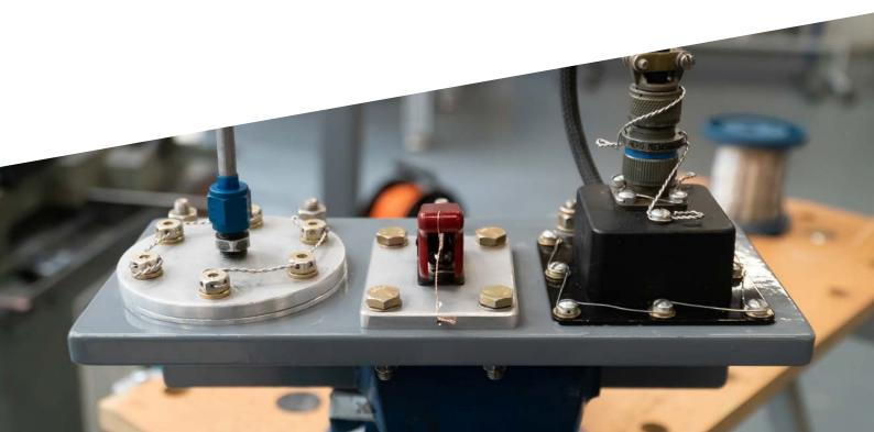
The Basic Flying Control Rod Trainer (BFCRT) provides basic training on flying control surface operations and adjustment and rigging of control systems.
