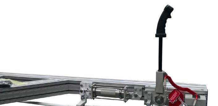
GenSkill is a freestanding physical representation of a typical Flying Control Run. The Generic Hand Skills Trainer (GenSkill) provides training in the hand skills necessary to work on aircraft components in confined spaces through access panels in an aircraft fuselage.
